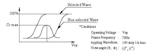
Contrast ratio (Cr) = <u>Brightness of selected dots</u> Brightness of non-selected dots
